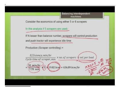
Now let us consider the economics of going for 5 scrapers. So, 5 in the sense you are going to use lesser than what is needed, you are assuming 5 that means you are going to use the number of scrapers lesser than what is needed. So, when the number of scrapers are lesser than the balanced number so obviously scrapers are more critical, but a pusher will have the ideal time. Your pusher will wait for the scraper.
